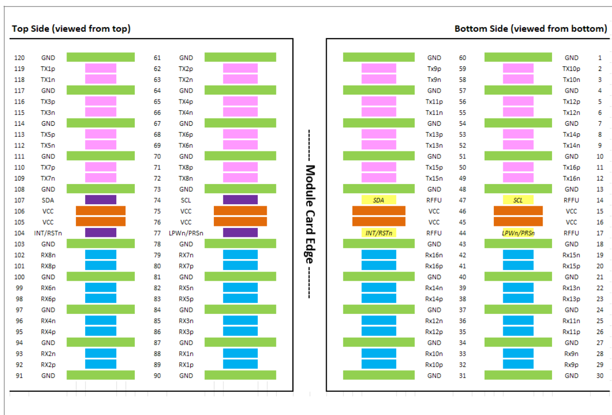
OSFP-XD Functional Pin Map (Module Perspective)
