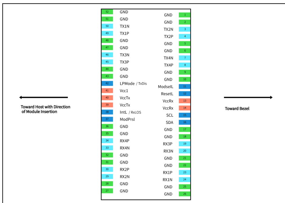
Figure 3 QSFP112 Host PCB pad assignment
