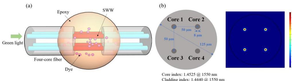
Fig. 1. (a) Schematic diagram of the SWW formed between four-core fibers; (b) Cross-sectional view and mode-field profile of the fiber.
