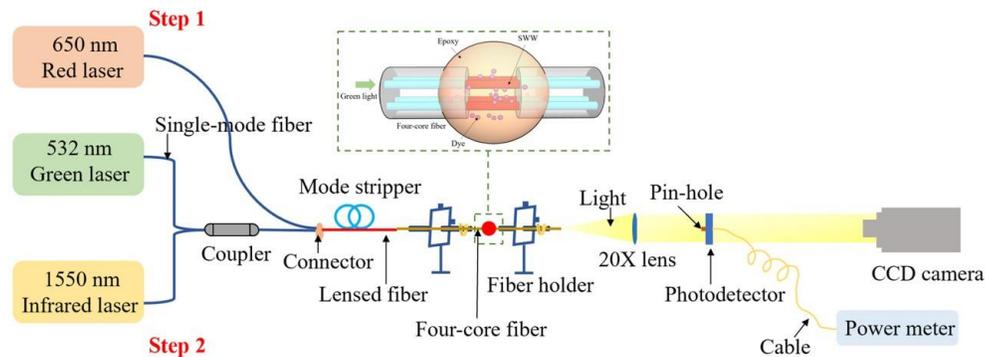
Fig. 2. Experimental setup. Initially, a CCD camera monitors the four-core fiber output light profile for optical path alignment. Subsequently, the CCD camera is replaced by a photodetector with a power meter to measure the output power at  $1550\ \text{nm}$  from the four-core fiber.
