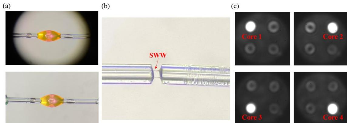
Fig. 3. (a) SWW forming process; (b) Microscopic image of the SWWs formed between two four-core fibers; (c) Output transmission mode of each core at a wavelength of  $1550\ \text{nm}$  after the SWW is formed.
