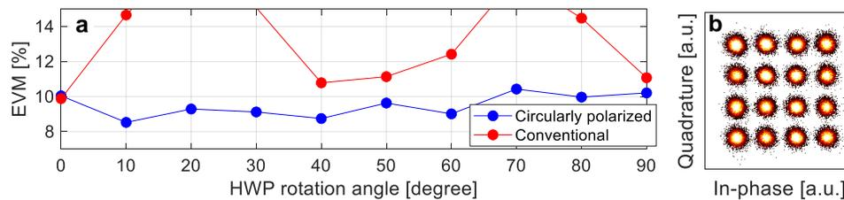
Fig. 4: a EVM dependence on angle rotation. b constellation plot of 25-Gbaud 16QAM.
