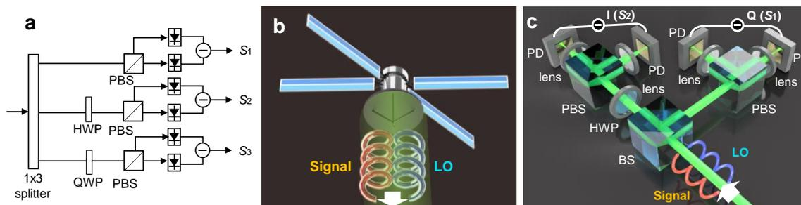
**Fig. 1:** a conventional standard SVR system. b illustration of circularly-polarized signal and LO waves emitted from a rotating satellite. c partial SVR enabling the IQ retrieval of the circularly-polarized self-homodyne signals.
