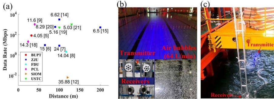
Fig. 1. (a) Recent long-distance demonstrations of UWOC systems, (b) a 2×2 MIMO-UWOC system in a swimming pool with air bubbles, and (c) the sea trial scene of the UWOC system based on beam-shaped LEDs.
