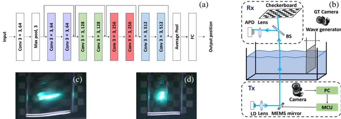
Fig. 1. (a) The structure of the ResNet-based model, (b) the experimental setup of the ResNet-based tracking system, and underwater camera captured images (c) with and (d) without wave.
