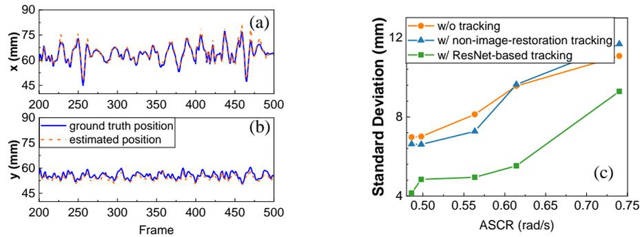
Fig. 2. Beam position estimation using trained ResNet-based model of (a) x- and (b) y-direction, and (c) standard deviation of beam positions versus wave average slope changing rate (ASCR).
