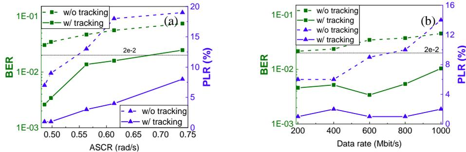
Fig. 3. BER and PLR performance without tracking and with ResNet-based tracking versus (a) ASCR with a 600-Mbit/s OOK signal and (b) data rate with a wave ASCR of 0.498 rad/s.
