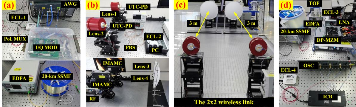
Fig. 2. Photos of setup: (a) optical transmitter, (b) THz wireless transmitter and receiver, (c) 3-m  $2 \times 2$  wireless link, (d) optical receiver.
