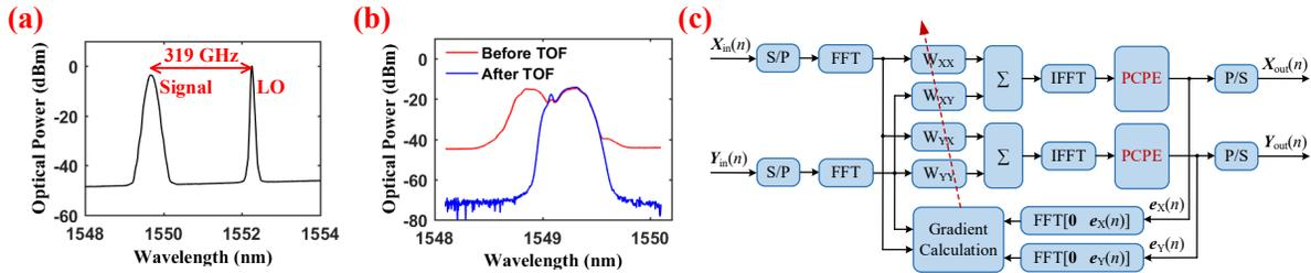
Fig. 3. (a) Optical spectra of optical signal and optical LO into UTC-PD; (b) Optical spectra of optical signals before and after TOF; (c) Block diagram of MIMO-FDE-PCPE algorithm.
