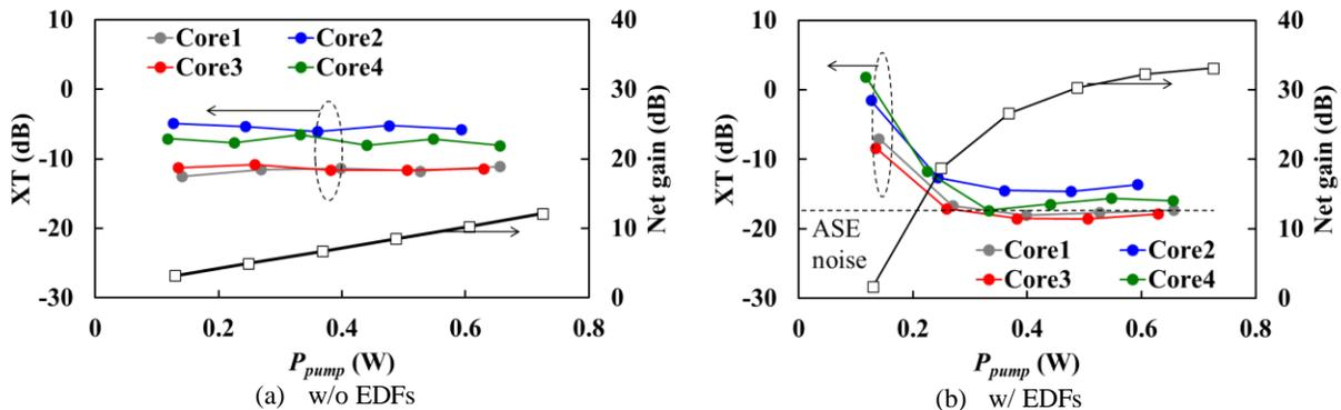
Fig. 3: Measured XT characteristics and net gain of unrepeated MCF link under counter-propagation
