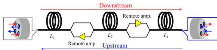
Fig. 1: Unrepeated MCF link under counter-propagation
