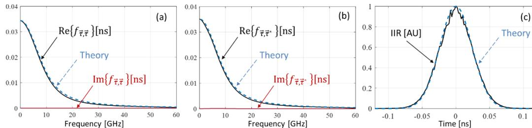
Figure 2 Real and imaginary parts of the correlation function of the complex-valued modal dispersion vector with (a) itself  $f_{\vec{\tau}, \vec{\tau}}$  and (b) with its complex conjugate  $f_{\vec{\tau}, \vec{\tau}^*}$ , and (c) the fiber intensity impulse response (IIR). Solid lines refer to the data and dashed lines to the theory.
