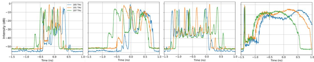
Figure 3 Intensity impulse response of the four FMF strands housed in the blue tube of the deployed FMF cable at the displayed frequencies (after [25]).
