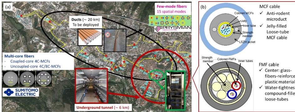
Figure 1 (a) SDM fiber testbed layout. The shorter ring of approximately six km is hosted in an underground tunnel network. The longer ring of approximately twenty km consists of traditional ducts. (b) Layout of the MCF (top) and FMF (down) cables.
