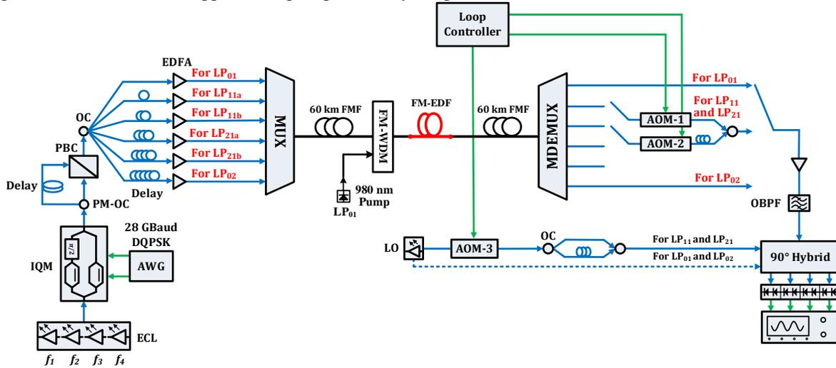
Fig. 4. Experimental setup of weakly-coupled MDM transmission with FM-EDFA.
