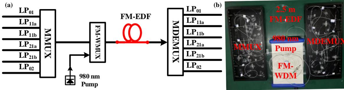
Fig. 2. (a) Experimental setup for 4-LP-mode FM-EDFA. (b) Picture of the experimental setup.
