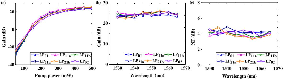
Fig. 3. (a) Gain versus powers of LP<sub>01</sub> mode pump. (b) Gain spectrum at the C band. (c) NFs at the C band.
