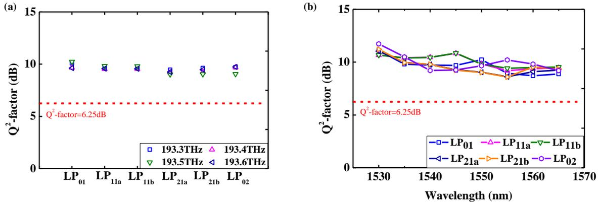
Fig. 5. (a) The  $Q^2$ -factors of 4-LP-mode MDM-WDM transmission over 60+60 km FMF. (b) The  $Q^2$ -factors versus wavelengths for MDM transmission at the C band.
