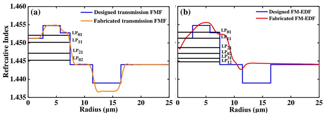
Fig. 1. (a) Index profiles of designed and fabricated transmission FMF. (b) Index profiles of designed and fabricated FM-EDF.
