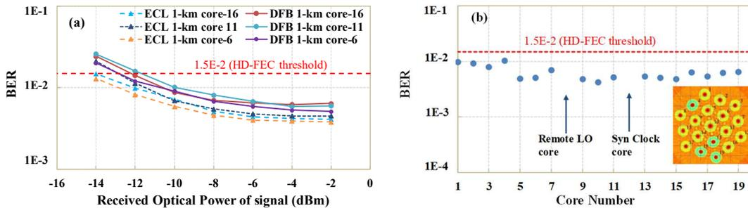
Fig. 4 (a) 1-km MCF BER vs ROP results for several channels under ECL and DFB cases, (b) BERs of all channels under DFB case.
