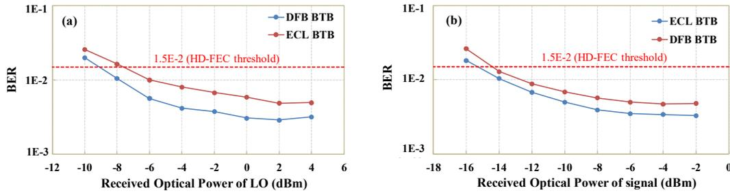
Fig. 3 BTB results for (a) BER versus received power of LO; (b) BER versus received power of signal with LO at 2 dBm.
