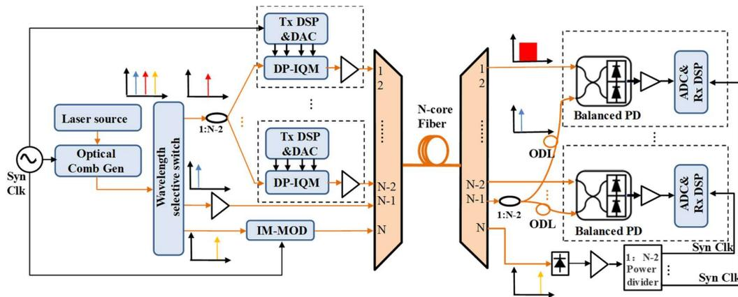
Fig. 1 Scheme of the proposed polarization-insensitivity self-heterodyne detection system.
