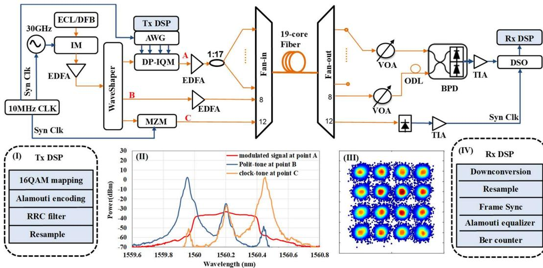
Fig. 2 experimental setup for 17×200-Gb/s transmission with self-heterodyne detection. (I) Tx DSP flow; (II) Optical spectrums of the modulated signal, pilot tone and clock-tone; (III) recovered constellation of 16QAM signal; (IV) Rx DSP flow.
