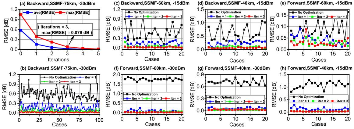
Fig. 2. (a) The variation of the average (blue) and the maximum (red) RMSE with optimization iteration in Sce. 2; (b)-(h) the RMSE of each case with optimization iterations of 0, 1, 2, and 3 in Sce. 2~Sce. 8.
