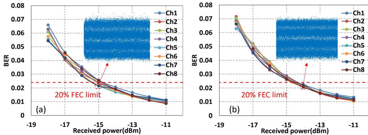
Fig. 4 Receiver sensitivity measured for the 8-ch PS-PAM-4 signals (a) BTB; (b) Connected via optical waveguide
