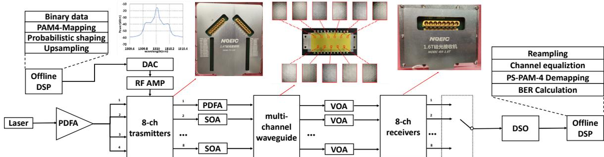
Fig. 2. Experimental setup for the interboard optical interconnection of 1.024-Tb/s PS-PAM-4 signals based on SiPh integrated transmitter and receiver array modules at O-band;
