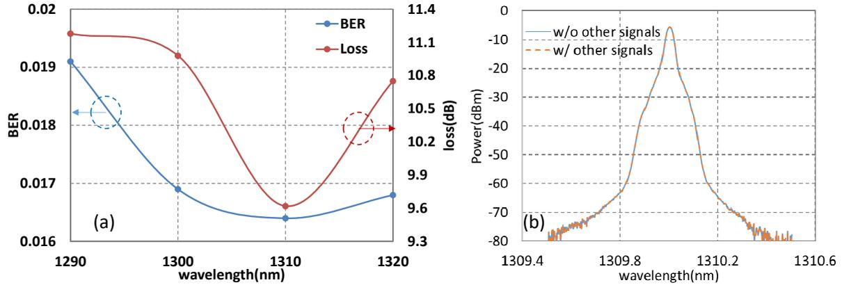
Fig. 3 (a) Measured curve of BER versus wavelength and Loss versus wavelength; (b) Signal spectrum with and without other channel signals
