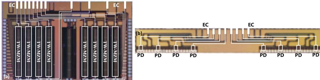
Fig.1 Optical micrograph of the 1×8 all-silicon transmitter (a) and receiver (b) array chip; EC, edge coupler; TW-MZM, traveling wave Mach-Zehnder modulator; PD, photodetector.
