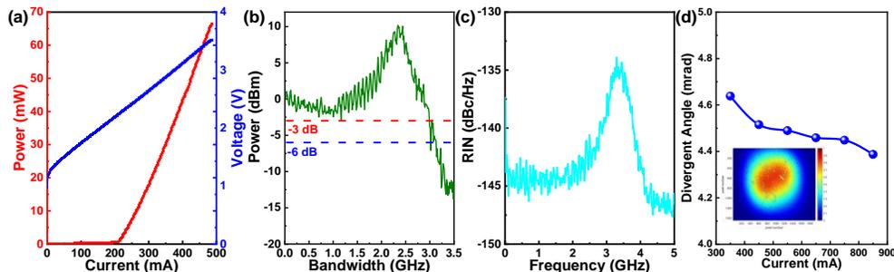
Fig. 2. (a) The  $P$ - $I$  and  $V$ - $I$  curves of the 940-nm PhCSEL operated under different DC biases; (b) the frequency response and (c) the RIN spectrum of the 940-nm PhCSEL operated under the  $2I_{th}$  condition; (d) the divergent angle of the 940-nm PhCSEL operated under different DC biases.
