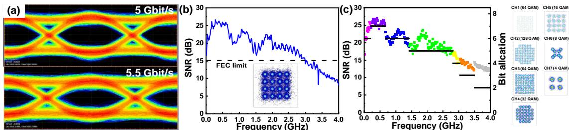
Fig. 3. (a) Eye-diagrams of the 5-Gbit/s and 5.5 Gbit/s NRZ-OOK data streams transmitted by the 940-nm PhCSEL. (b) SNR spectrum and constellation plot of the 4-GHz 16-QAM DMT data stream transmitted by the 940-nm PhCSEL. (c) SNR spectrum and corresponding constellation plots of the bit-loaded DMT data stream transmitted by the 940-nm PhCSEL.
