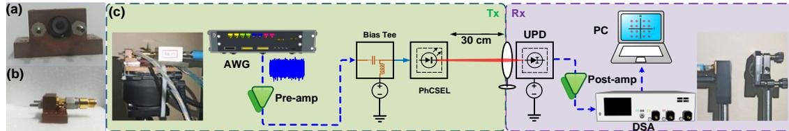
Fig. 1. (a) Photograph of the 940-nm PhCSEL; (b) Photograph of the laser package; (c) Photograph and schematic diagram of the testing transmission system of the short-reach FSO data link.
