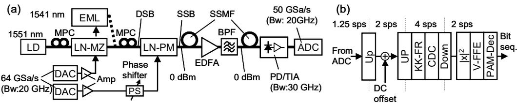
Fig. 3. Schematic diagram of (a) setup and (b) receiver-side DSP of IM/DD 40-GBaud polar-coordinate SSB PAM4 transmission experiments. MPC: manual polarization controller, BPF: Optical band-pass filter, SMF: Standard single-mode fiber, KK-FR: Field reconstruction by KK method, CDC: CD compensation, V-FFE: Volterra non-linear FFE.
