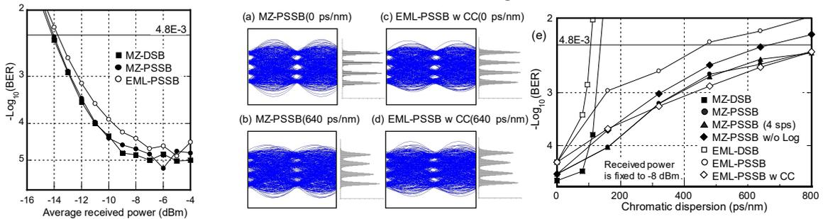
Fig. 5. Back-to-Back BER curves of IM/DD 40-GBaud MZ-DSB, MZ-PSSB and EML-PSSB PAM4 signals.
