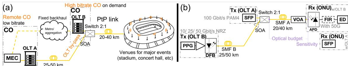
Fig. 1. (a) Scenario studied and (b) Experimental setup with bypass of OLT-A
