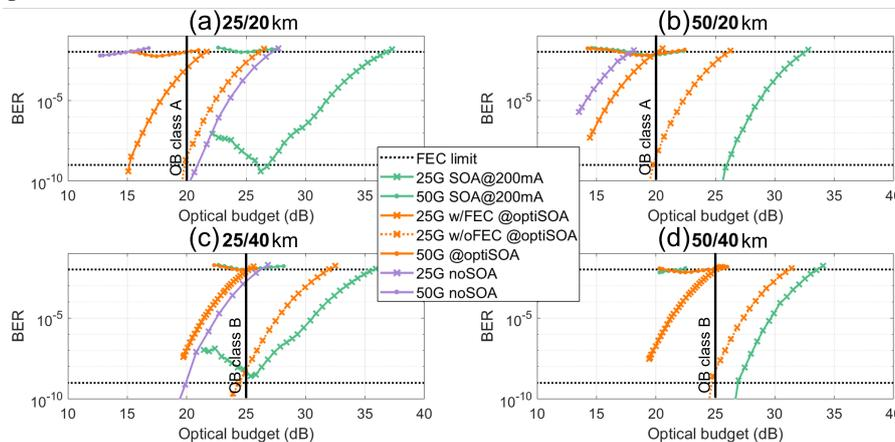
Fig. 2. BER curves for various distances, presented with two bitrates (25 Gbit/s and 50 Gbit/s NRZ) and with three different configurations: SOA at 200 mA, optimised SOA current and no SOA
