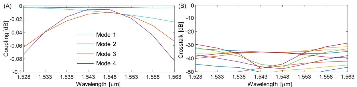
Figure 2 – (A) IL of four-mode spatial multiplexer across C-band. (B) Modal crosstalk to other modes than target.
