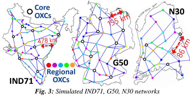
Fig. 3: Simulated IND71, G50, N30 networks
