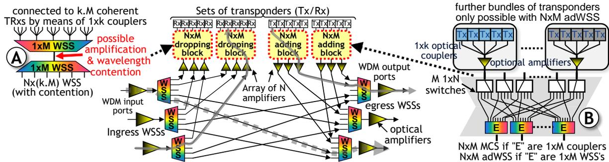
Fig. 1: 3-degree WSS-based OXC equipped with CD ADBs (A) or CDC ADBs (B). If the E components in CDC ADBs are 1xM couplers (resp. 1xM WSS's,) then modules B are MCS's (resp. adWSS's). Tx: transmitter. Rx: Coherent receiver.
