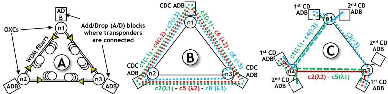
**Fig. 2:** (A) 3-node triangle network topology; (B) possible wavelength allocation without add/drop constraint; (C) wavelength allocation with CD constraint in ADBs and gradual deployment of ADBs leading to suboptimal network performance.
