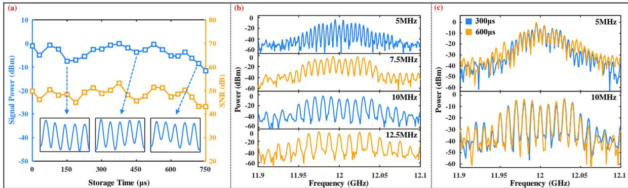
Fig. 3. (a) Power and SNR changes of the 12 GHz signal during storage. (b) The beat signal spectra of the Doppler-frequency modulated carriers and the RF-modulated signal before storage, with the Doppler frequencies of 5, 7.5, 10, and 12.5 MHz. (c) The beat signal spectra of the Doppler-frequency modulated carriers and the RF-modulated signal after 300  $\mu\text{s}$  and 600  $\mu\text{s}$  storage, with the Doppler frequencies of 5 and 10 MHz.
