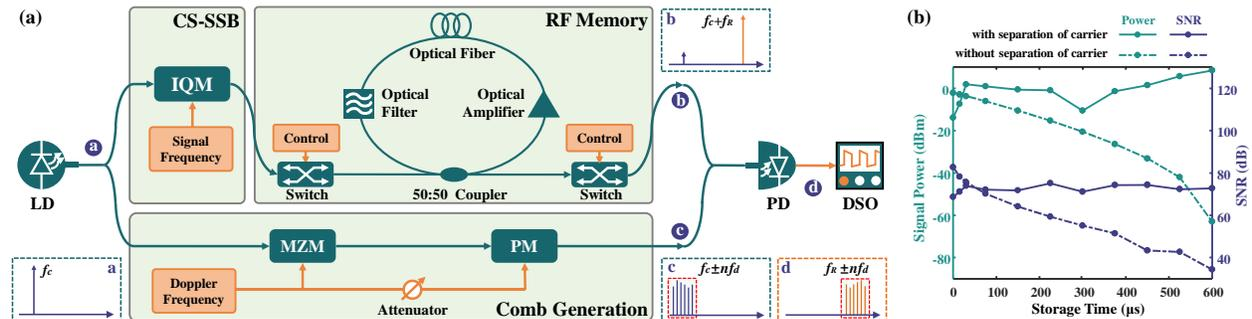
Fig. 1. (a) Experimental setup of the frequency-comb-enabled PRFM system for multi-false-target radar compound jamming. (b) Simulated power and SNR changes of a stored 20 GHz signal in different schemes.
