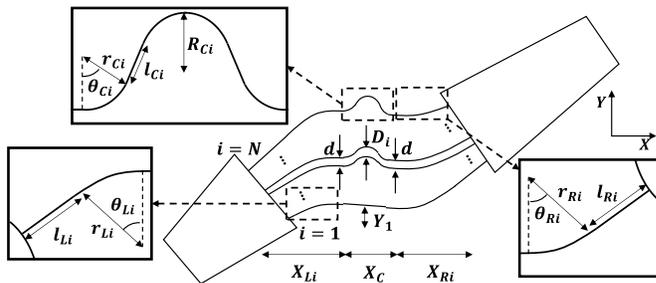
Fig. 2 Proposed design of the small-footprint arrayed waveguide grating.
