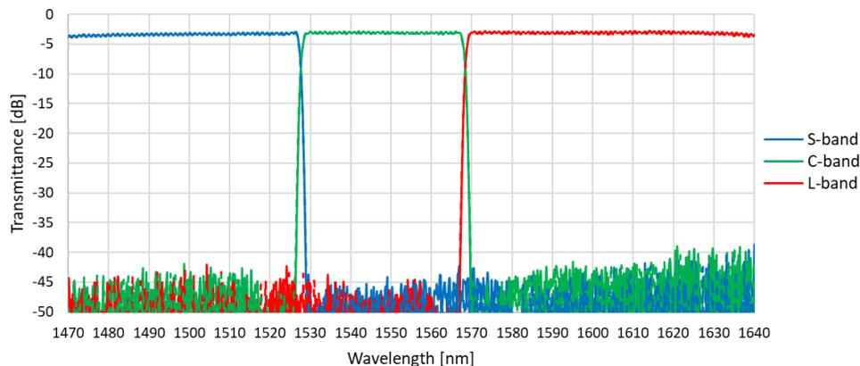
Fig. 4 Experimental results of the transmission spectrum of the fabricated waveband MUX/DEMUX filter using the compact cascaded AWGs. The solid line is drawn in TM mode and the dashed line in TE mode; these lines overlap due to the small polarization dependence (polarization dependent loss  $< 0.3 \text{ dB}$ ).
