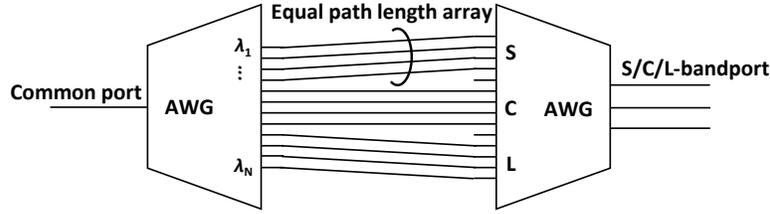
Fig. 1 Schematic illustration of a SCL-band MUX/DEMUX filter using cascaded AWGs.
