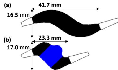
Fig. 3 Design comparison between (a) S-shape and (b) proposed AWGs using common AWG parameters. In (b), the waveguides in the center block are drawn in blue.
