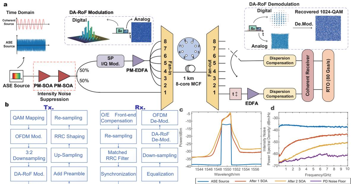
Fig. 1. (a) Experimental setup, (b) DSP procedure, (c) Spectrum and (d) Intensity Noise Power Spectral Density of ASE source without SOA, with 1 SOA and with 2 SOAs. The purple line is PD noise floor.
