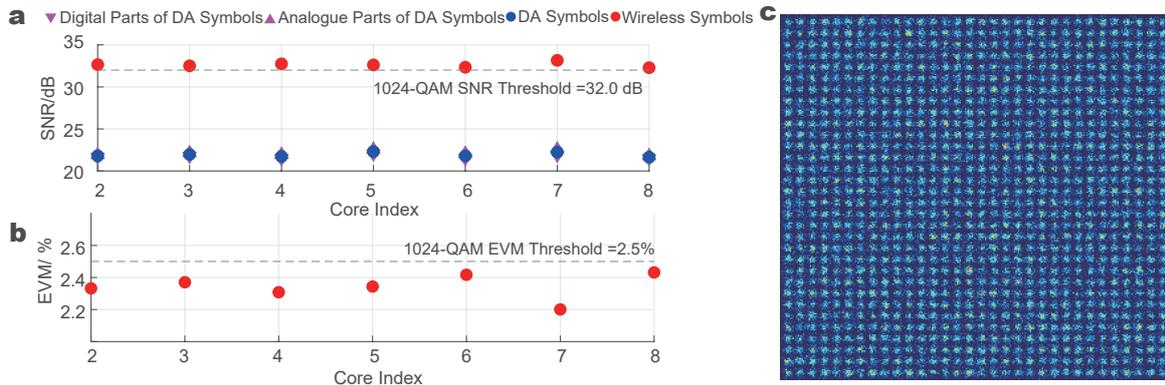
Fig. 3. (a) SNR of digital and analog parts of DA symbols, recovered wireless symbols and (b) EVM of all MCF cores used for transmission. (c) the constellation of the recovered 1024-QAM wireless signal of core 7.
