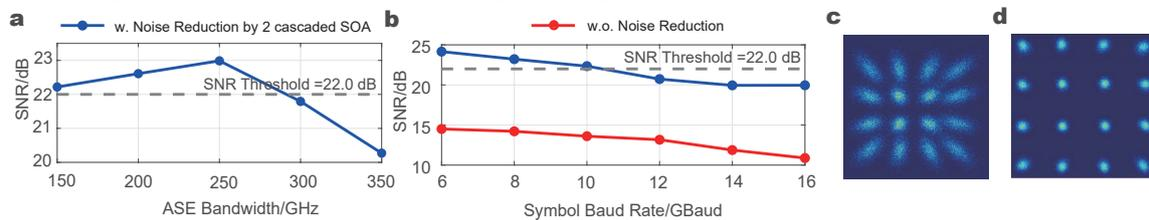
Fig. 2. (a) SNR versus ASE bandwidth of 16-QAM coherent signal of Core 4, (b) SNR versus symbol baud rate of Core 4, and 16-QAM constellation (c) without SOA and (d) with 2 cascaded SOAs.
