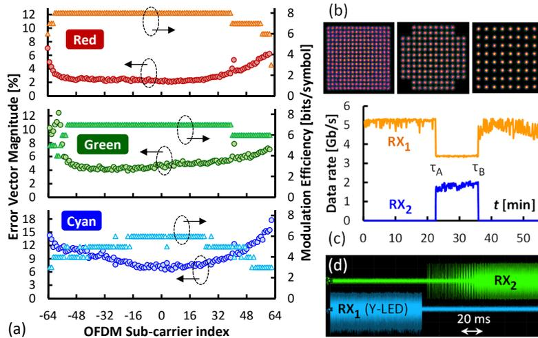
Fig. 3. (a) EVM and spectral efficiency for pencil beam reception and (b) constellations for the red WDM channel. (c) Aggregated WDM rates and (d) received signal when switching of the green channel between the two receivers.
