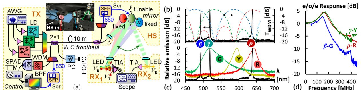
Fig. 1. (a) Experimental setup. (b) Optical emission of LDs and WDM channels. (c) Spectral allocation and (d) e/o/e link response of LD-LED pairs.
