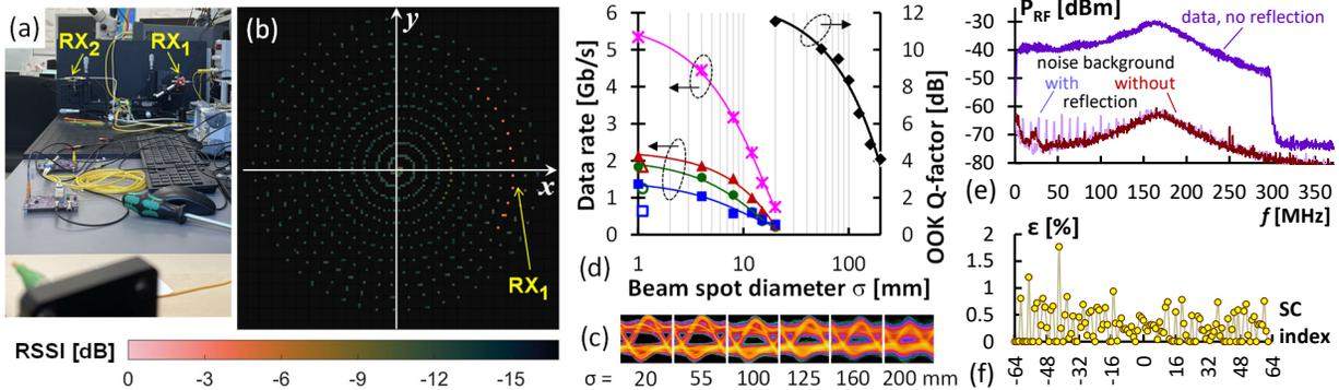
Fig. 2. (a) View on LED receivers from the hotspot and (b) spiral-search of receivers emitting a beacon. (c) Wide-beam OOK eye diagrams. (d) Supported OFDM rates and OOK Q-factor for narrowed beam. (e) Received RF spectrum in presence of reflections and (f) EVM penalty.
