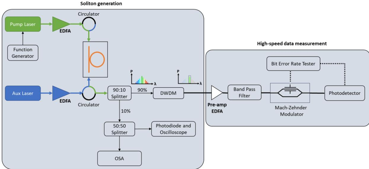
Fig. 1. Schematic of the experimental setup used in this work. EDFA: Erbium-Doped Fiber Amplifier, DWDM: Dense-Wavelength Division Multiplexer.
