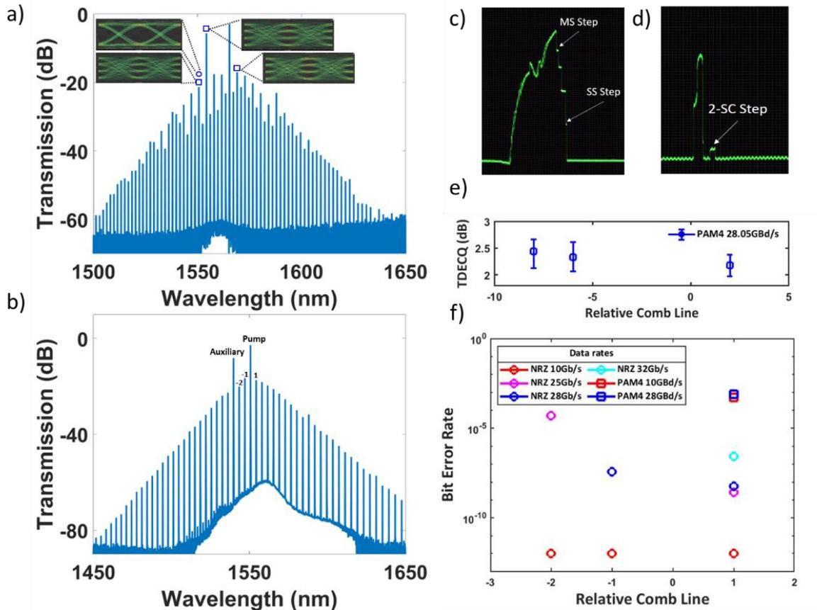
Fig. 2. Spectra of the microresonator-based generation of a) multi-soliton (MS) state b) 2-soliton crystal (SC) state. The inset shows the measured eye diagrams corresponding to data modulated on the labelled frequency comb lines.
