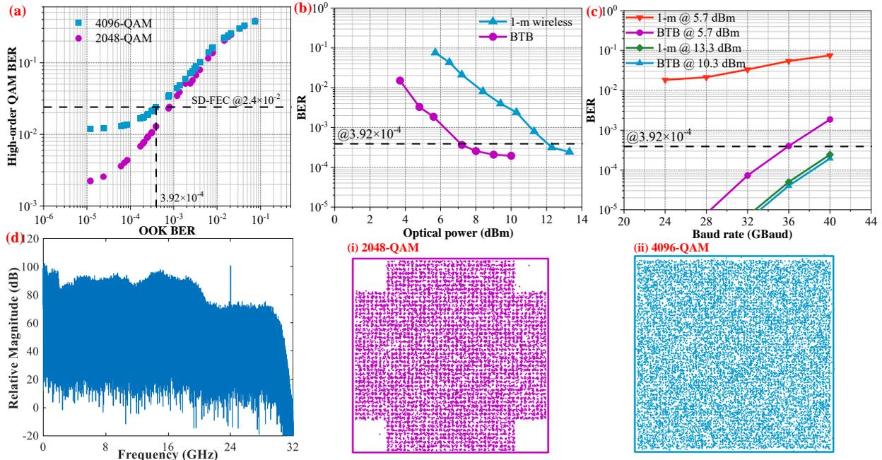
Fig. 2. The experimental results. (a) BER curves of the recovered high-order QAM versus the BER of the DSM-OOK signals; Measured BER of the DSM-OOK with (b) different optical power and (c) different baud rate; (d) Spectrum of the received baseband signal after 1-m wireless transmission; Constellations of the recovered (i) 2048-QAM and (ii) 4096-QAM.
