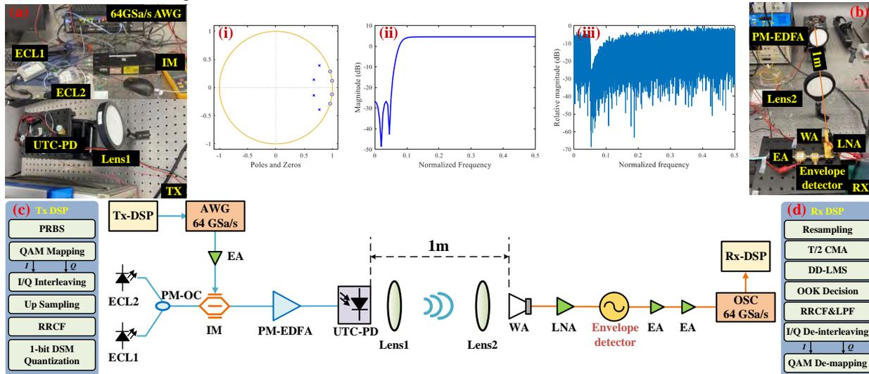
Fig. 1. Experimental setup of the THz communication system using DSM in IM/DD channel. Photos of (a) transmitter; (b) transmission link and receiver. (c) Tx DSP; (d) Rx DSP.
