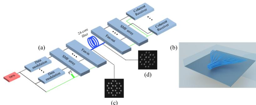
Fig. 1. (a) Conceptual illustration of SDM-SHD system of a 2.7km 24-core SM-MCF; (b) Concept of the femtosecond laser inscribed on-chip FIFO device; (c) the output light field intensity profile of FIFO device; (d) the output light field intensity profile of 24-core SM-MCF.
