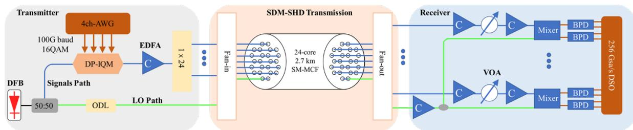
Fig. 2. Experimental configuration of transmitting 102-Gbaud DP-16QAM signals over a 24-core SM-MCF in the SDM-SHD system. ODL: Optical delay line. DP-IQM: dual-polarization IQ modulator. AWG: arbitrary waveform generator. EDFA: erbium-doped fiber amplifier. VOA: arbitrary waveform generator.
