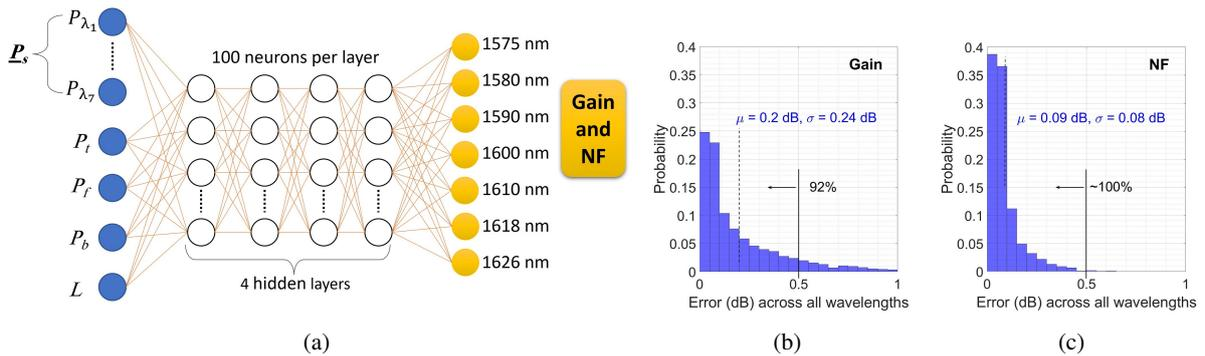
Fig. 2: a) The FFNN structure, and histograms of the absolute error in dB for b) gain, and c) NF prediction.
