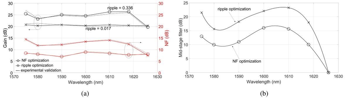
Fig. 3: a) Gain (solid lines) and NF (dashed lines) vs. wavelength for two optimizations, and b) corresponding mid-stage band pass filters for the two optimizations.
