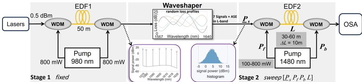
Fig. 1: Experimental setup for capturing the training and test sets (OSA: optical spectrum analyzer). The waveshaper has four examples from the random loss profiles we applied; insets are for fixed output spectrum of Stage 1, and a histogram of total power input to Stage 2 when using the random loss profiles.
