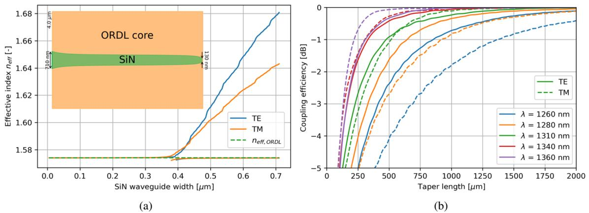
Fig. 2: Lumerical Mode simulation results: (a) The guided mode's effective index varies along SiN width variations; the inset shows the optimal taper shape, (b) SiN-to-ORDL coupling efficiency displays the desired adiabatic behaviour for different O-band wavelengths as function of the taper length.
