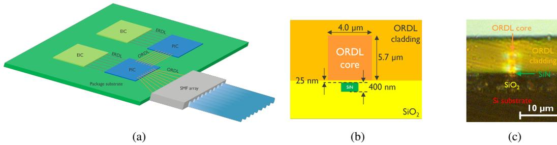
Fig. 1: Visualisation of the SiN-to-ORDL configuration: (a) SiN (tapered) waveguides are located on the embedded PIC(s), while the ORDLs connect the PIC to another PIC and SMF array, (b) Schematic cross-section, including target dimensions, (c) Microscope image indicating all present materials.
