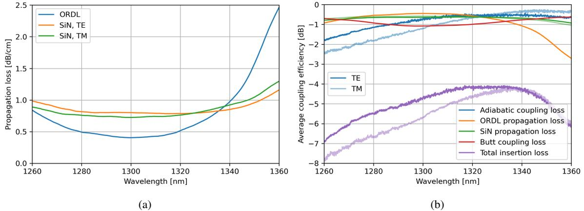
Fig. 3: (a) Propagation loss for SiN and ORDL, (b) Average optical performance for all individual loss contributions are shown, as well as the total insertion loss. Note that the total insertion loss equals two times butt-coupling, ORDL and SiN propagation loss and two times adiabatic coupling loss for 1 mm long "Monotonic mode tracking" (Mono) tapers.
