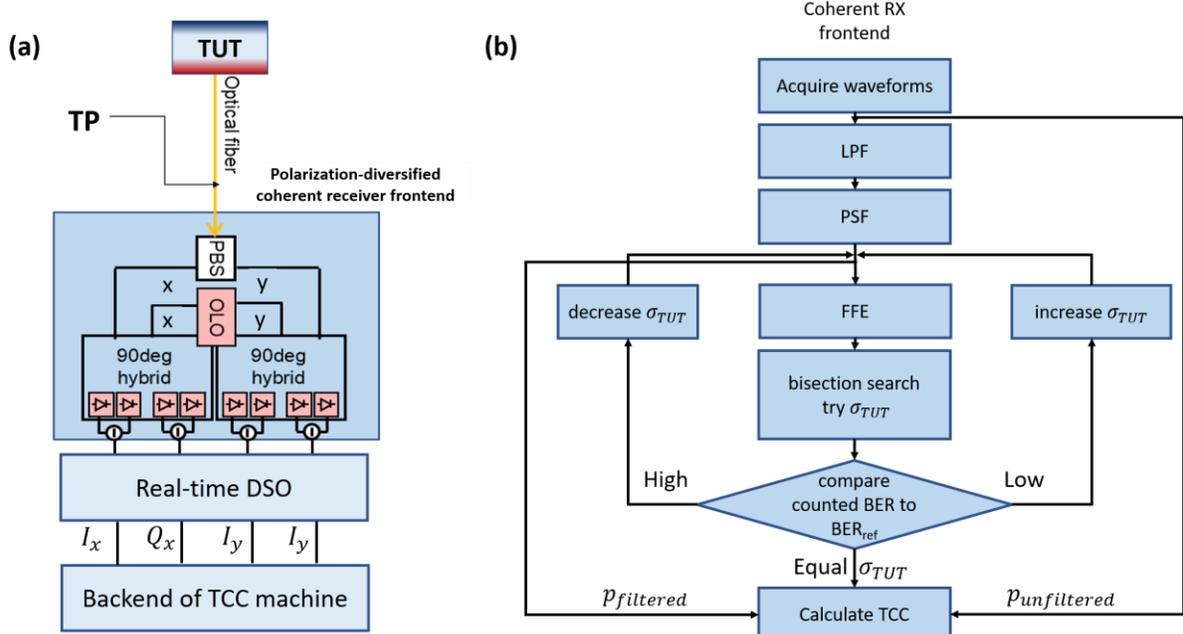
Fig. 1. TCC scheme. (a) A reference optical coherent frontend of TCC machine acquires the signal sent from transmitter under test (TUT) at test point (TP). DSO: digital oscilloscope. (b) flowchart of the TCC machine backend. Constellations are recovered by reference DSP, where a noise search loop is conducted to measure the noise tolerance to reach target  $BER_{th}$ , along with power adjustment, giving rise to TCC result.
