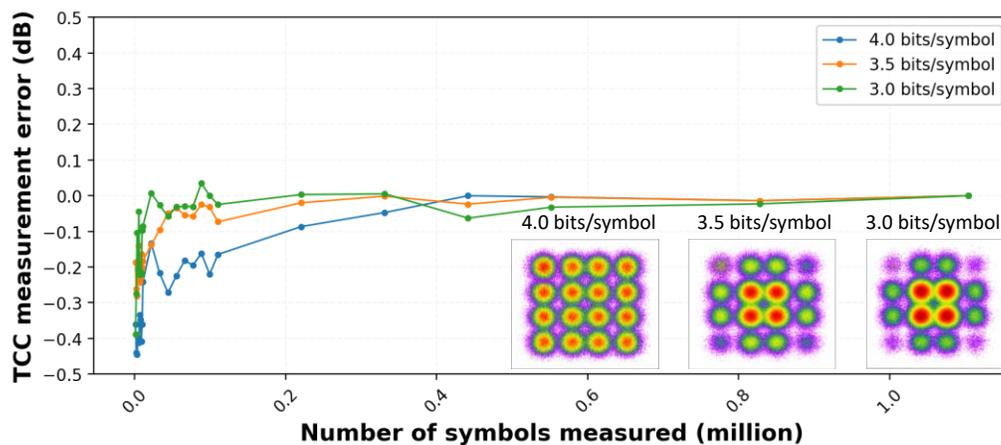
Fig. 3. TCC measurement error at  $BER_{th}=1E-2$  for DP-16QAM and PCS-shaped DP-16QAM.
