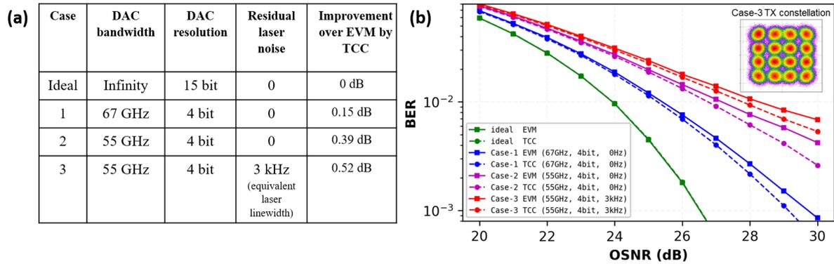
Fig. 2. Simulation setup: 125GBaud, up shaped DP-16QAM, PCS: 4, 3.5, or 3 bits/symbol, 0 roll-off RC, ideal reference receiver, over 1 million symbols measured for each case,  $BER_{th}=1E-2$ . (a) simulation cases (b) BER versus OSNR for the four cases measured by the EVM and TCC metrics.
