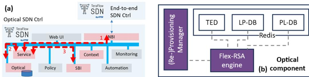
Fig. 1. (a) TeraFlowSDN-based Optical SDN controller and workflow; (b) Optical component.
