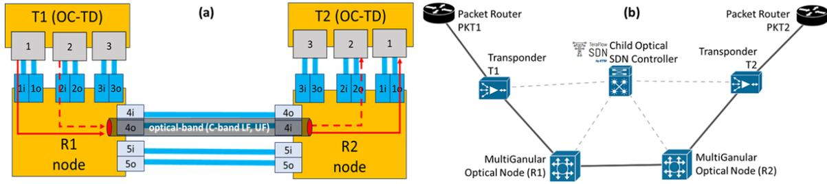
Fig. 2. (a) Scenario of an optical-band; (b) Topology view at End-to-end SDN controller.
