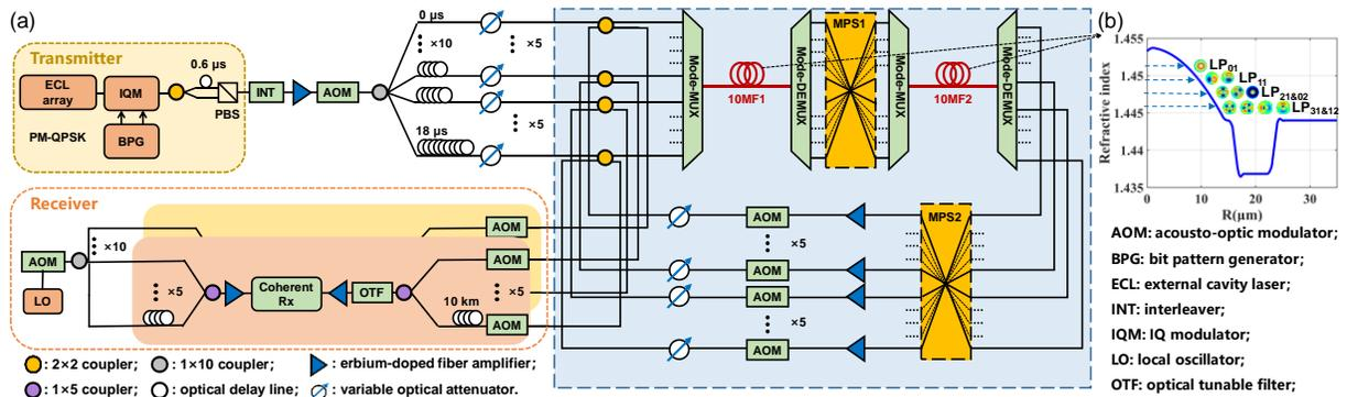
Fig. 2. (a) Experimental setup for the 10-mode joint mode-permuted transmission. (b) The refractive index profile of the fabricated 10-mode fiber and the corresponding guided modes.
