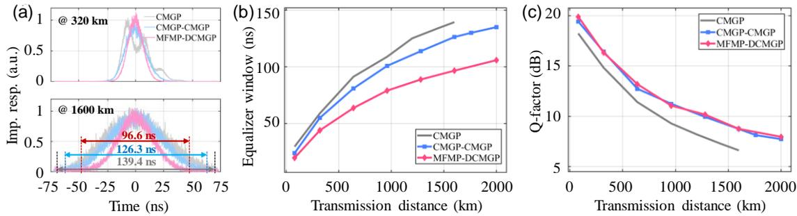
Fig. 3. (a) Impulse responses for different mode permutation schemes observed at 320 km and 1600 km, respectively. The required equalizer windows (b) and Q-factors (c) as functions of transmission distance for different mode permutation schemes. Compared with the conventional CMGP, the required equalizer window is further reduced by 30.7%, while the transmission reach is extended to 2000 km, increased by 400 km.
