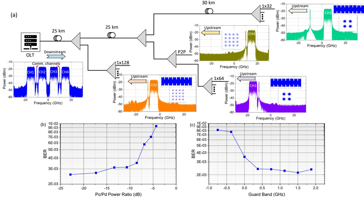
Fig. 3. (a) Experimental setup; (b) Subcarrier BER versus Pc/Pd power ratio; (c) Subcarrier BER versus guard band size.
