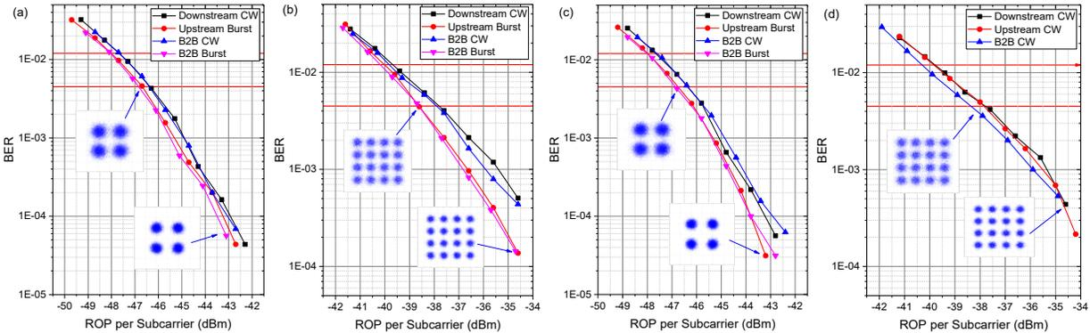
Fig. 4. Experimental results for downstream and upstream transmission: (a) BER versus ROP in subcarrier 1; (b) BER versus ROP in subcarrier 2; (c) BER versus ROP in subcarrier 3; (d) BER versus ROP in subcarrier 4.
