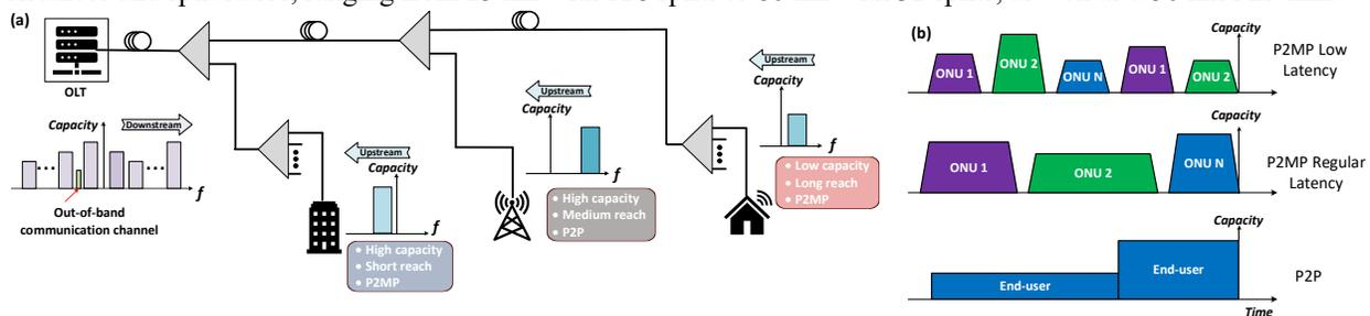
Fig. 1. (a) Coherent TFDM PON featuring adaptive capacity and distributed splitting; (b) TFDM subcarriers support various services with different capacity and latency requirements.
