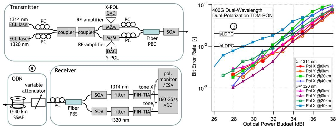
Fig. 2. Experimental setup to validate 400G DW-DP PON (a). Measured BER versus received optical power for the four channels for different fiber reaches (b).
