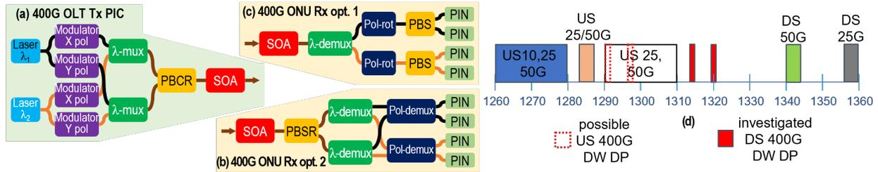
Fig. 1. 400G DW-DP transmitter (a) and receiver options (b,c). Pol rot – polarization rotator, pol demux – polarization demultiplexer. (d) XG(S), 25G and 50G PON wavelength plan with proposed wavelengths for 400G DW-DP PON.
