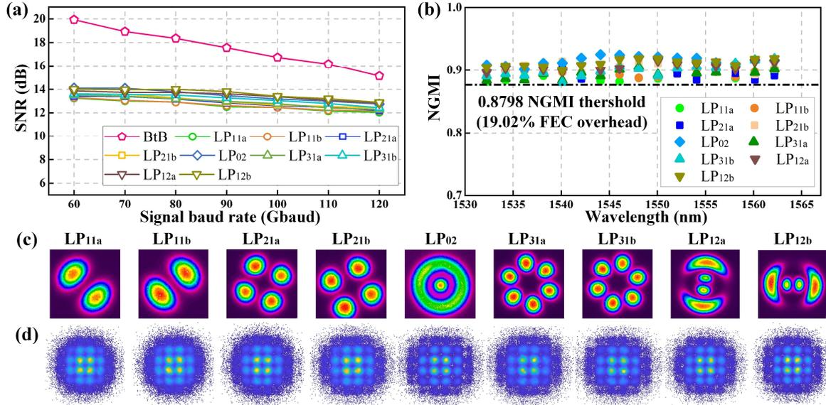
Fig. 3 Performance of the MDM-SHCD system. (a) Measured SNR versus baud rate of signal. (b) NGMI performance of 120-Gbaud PCS-64-QAM signals in the 9 mode channels at 16 wavelengths. (c) Mode patterns at 1550 nm after 30-km FMF transmission. (d) Recovered PCS-64QAM constellations of the 9 mode channels at 1550-nm wavelength.
