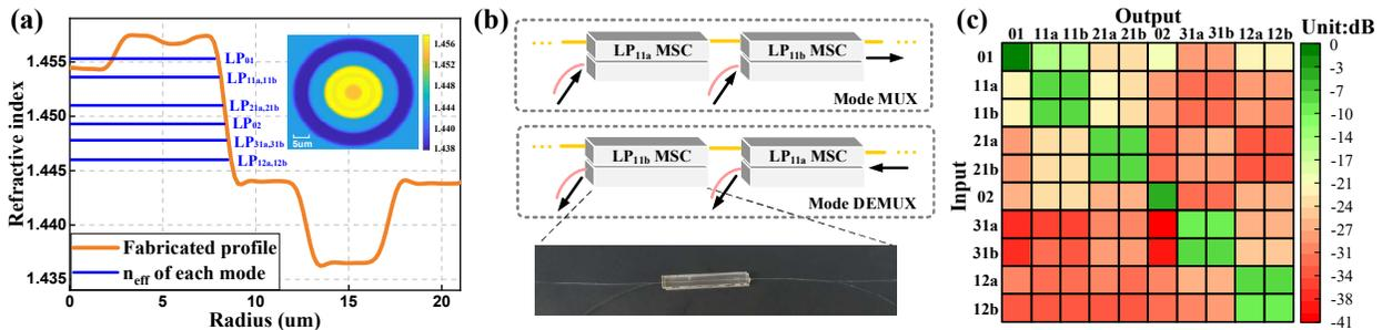
Fig. 2 (a) Index profile of the fabricated weakly-coupled MRC FMF supporting 10 modes (6 LP modes). (b) Cascaded structure diagram of the mode MUX/DEMUX. (c) Normalized crosstalk matrix at 1550 nm.
