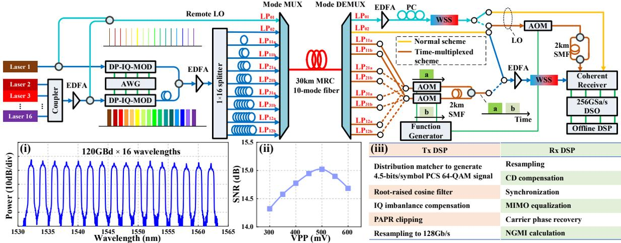
Fig. 1 Experimental setup for the high-capacity MDM-SHCD transmission. Inset (i) Measured optical spectrum of the transmitted WDM signal. (ii) Back-to-back (BtB) signal SNR versus AWG output swing. (iii) DSP algorithms employed for transmitter and receiver. SNR: signal-to-noise ratio; PAPR: peak-to-average-power ratio; CD: chromatic dispersion.
