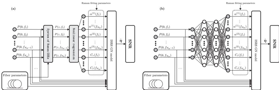
Fig. 1: Schematics for SNR prediction using ISRS GN model with  $f$ -dependent parameters  $C_r(f_k)$ ,  $\alpha^{(1)}(f_k)$  and  $\alpha^{(2)}(f_k)$  in Eq. (2) by (a) numerically solving Raman ODEs followed a nonlinear regression and (b) a fully-connected DNN.
