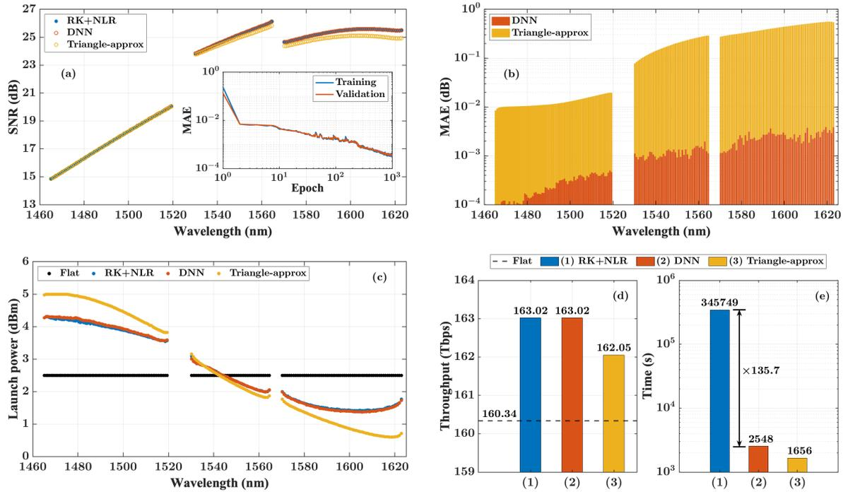
Fig. 2: Performance evaluation of RK+NLR, proposed DNN, and triangle-approximation on: (a) mean SNR per channel of the validation dataset; (b) MAE of the mean SNR with respect to the labeled dataset; (c) flat and optimized launch power profiles by PSO and (d) their corresponding achieved throughput and (e) computational time.
