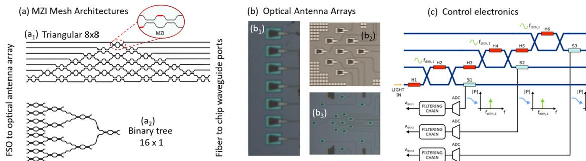
Figure 1. (a) Schematic of the MZI-based photonic processors with triangular and binary-tree topologies. (b) Top view photograph of on-chip optical antenna made of 1D linear (b<sub>1</sub>), 2D square (b<sub>2</sub>) and 2D circular array (b<sub>3</sub>) of GCs; (c) Scheme of the control electronics for automated configuration and stabilization of the cascaded MZIs of the integrated photonic processors.
