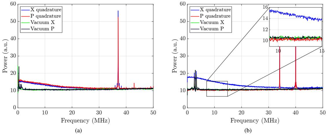
Fig. 2: Spectrum of the signal before and after the DSP procedure. (a) Detected signal before frequency and phase recovery (b) Signal after phase recovery (Inset: frequency range under investigation)
