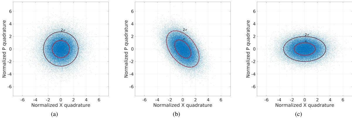
Fig. 3: State ensemble. (a) Before phase recovery; (b) After phase recovery; (c) After quadrature remapping
