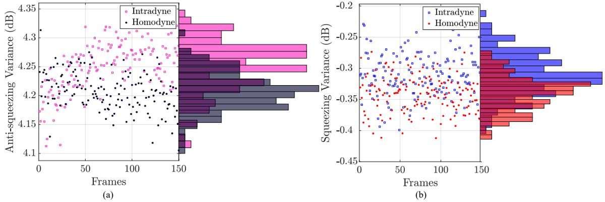
Fig. 4: Squeezed light measurement using carrier phase recovery in comparison with conventional homodyne detection. Each frame consists of  $8 \times 10^4$  symbols.
