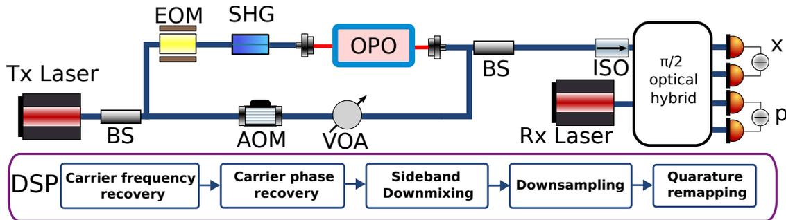
Fig. 1: Experimental setup and digital signal processing (DSP) routine. EOM: electro-optics modulator, SHG: second-harmonic generator, OPO: optical parametric oscillator, AOM: acousto-optics modulator, VOA: variable optical attenuator, BS: beamsplitter, ISO: optical isolator.
