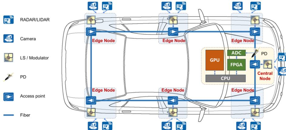
Fig. 1. An exemplary system block diagram of an intra-vehicle optical network.
