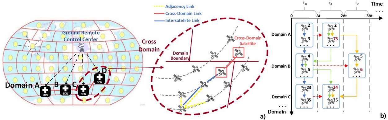
Fig. 1. (a) The link diagram of distributed sequence routing based on geographic location division of control plane is established. (b) Domain-sequential routing sequence switching.
