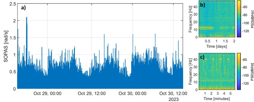
Fig. 2. a) 4 days SOPAS time evolution, b) 2 days  $S_3$  spectrogram, c)  $S_3$  spectrogram when inducing 40 Hz mechanical vibrations on the fiber. Metropolitan fiber is always considered for these plots.
