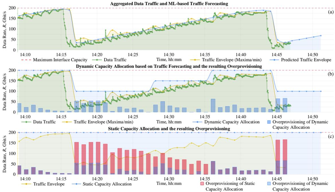
Fig. 2. Grafana dashboard for demonstration of dynamic link-capacity allocation: (a) Example of aggregated bursty and cyclic traffic with a 3s traffic sampling granularity, its traffic envelope, and predicted envelope/traffic evolution. (b) Dynamic link-capacity allocation and the resulting over-provisioning. (c) Static/fixed link-capacity at 200G, and the comparison of over-provisioning amounts for dynamic vs. static capacity allocation schemes.
