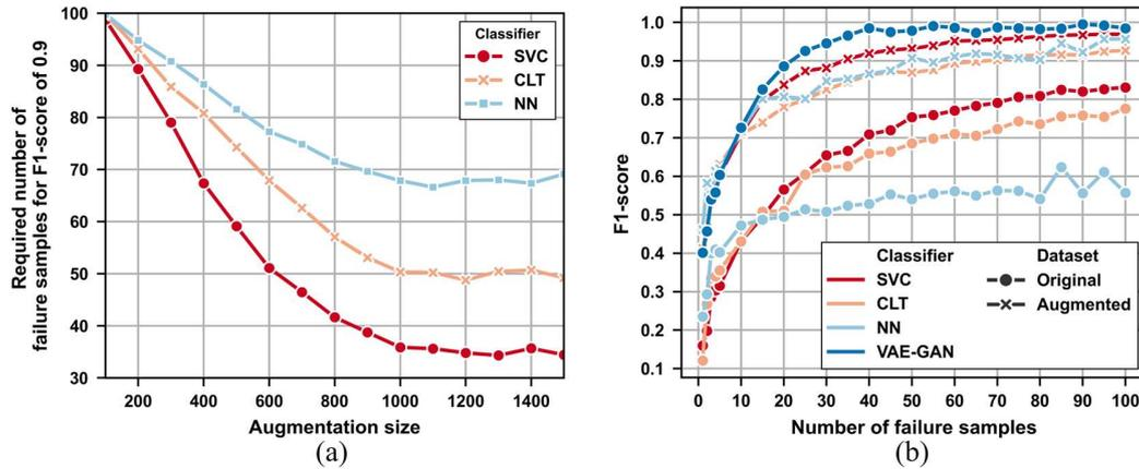
Fig. 2. (a) Required number of real failure samples to reach an F1-score of 0.9 over the augmentation size from those samples; (b) F1-score over number of failure samples used to train the VAE and the GAN for data augmentation with an augmentation size of 1000; SVC: Support vector machine-based classifier, CLT: Classification tree, NN: Neural network
