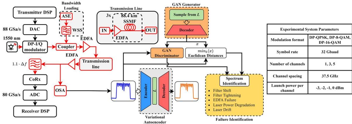
Fig. 1. Experimental setup and data augmentation chain with a generative adversarial network (GAN) and a Variational Autoencoder (VAE) for soft-failure identification,  $L$ : latent space; DAC: digital-to-analog converter, ASE: amplified-spontaneous emission, WSS: wavelength selective switch, EDFA: Erbium-doped fiber amplifier, SSMF: standard single-mode fiber, OSA: optical spectrum analyzer, ADC: analog-to-digital converter, DSP: digital signal processing.
