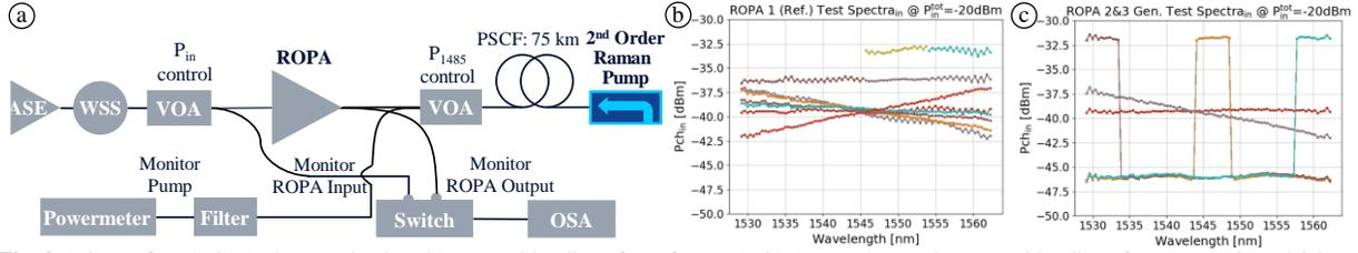
Fig. 2 a) Setup for a ROPA characterization, b) spectral loadings for reference ROPA test, c) generic spectral loadings for target ROPA 2&3 test.
