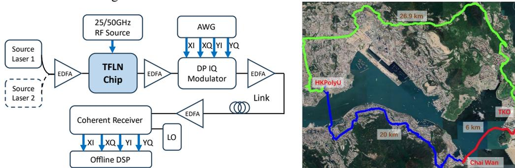
Fig. 2. WDM transmission experimental setup and the route of the field-deployed link across Hong Kong.
