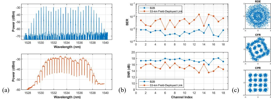
Fig. 3. (a) Spectrum of the  $50\text{ GHz}$  EO comb and corresponding WDM signal; (b) SNR and BER of the  $50\text{ GHz}$  EO comb WDM signal for B2B and  $53\text{-km}$  field-deployed link transmission. (c) Received signal distributions at various stages of receiver DSP.
