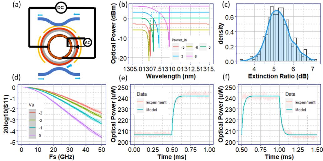
Fig. 2 Model-hardware correlations for: (a) a cartoon of GF Si MRM; (b) ring modulator transmission curve with bistable states at different power (-6,-3,0,3,6)dBm. (c) Micro-ring modulator extinction ratio at minimum transmission penalty; (d) Model hardware correlation: S11 parameter of ring PN junction with open-short deembedding. (e)(f) Thermal constant characterization (heating and cooling transient).
