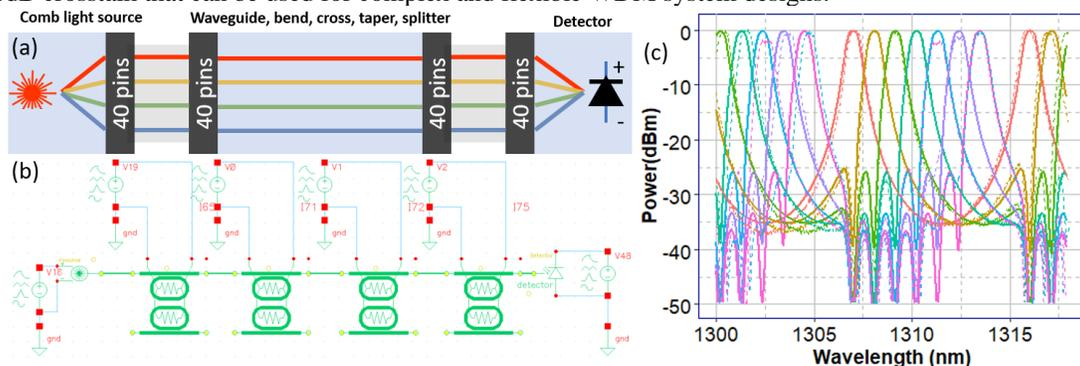
Fig. 3. (a) 4-channel light-source, waveguide and photodetector schematic as an example of multichannel enablement; (b) Schematic of the 4-channel WDM; (c)  $8\lambda$  model-hardware correlation: with adjustable flatness, channel spacing and channel width (model: solid; hardware: dashed).
