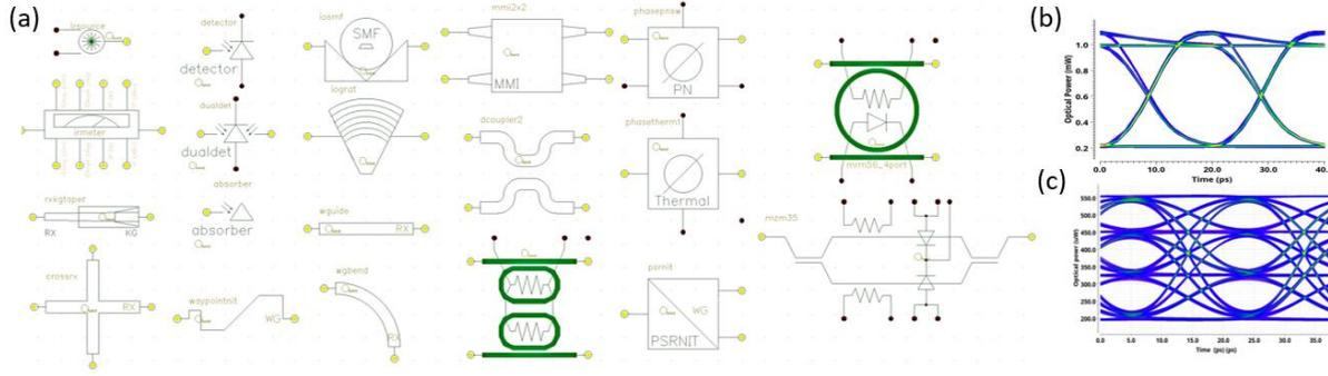
Fig. 1. (a) Passive and Active device library including I/Os, phase shifters, detectors, couplers and EO modulators; (b) high-power MRM dynamic simulation: the eye-diagram of 53Gb/s PRBS at 3dBm; (c) MZM simulation: The eye-diagram of 53Gb/s PAM4.
