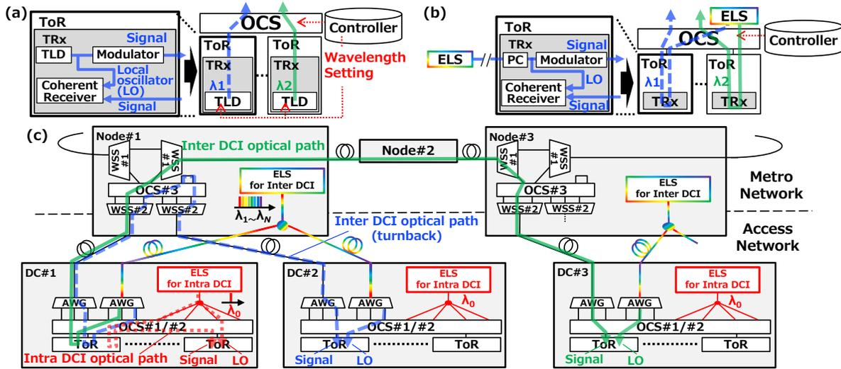
Fig. 1: Wavelength settings and optical-path routing schemes in OCS-based DCs. (a) With conventional digital coherent TRx. (b) With digital coherent TRx used in proposed DCN. (c) Proposed converged all-optical intra/inter DCN.
