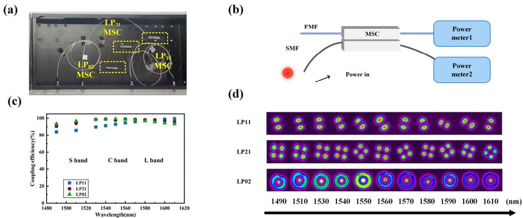
Fig. 2 (a) The picture of the fabricated MSCs. (b) The experimental setup for coupling efficiency measurement. (c) The measured coupling efficiency of each mode across 1490~1610 nm. (d) Measured mode fields across 1490~1610 nm.
