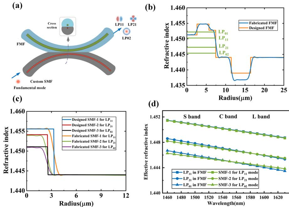
Fig. 1 (a) Schematic structure of a MSC with side-polishing processing. (b) Index profiles of designed and fabricated MRC-FMF. (c) Index profiles of designed and fabricated custom SMFs. (d) Calculated  $n_{\text{eff}}$  of fabricated custom SMFs and high-order LP modes of fabricated MRC-FMF.
