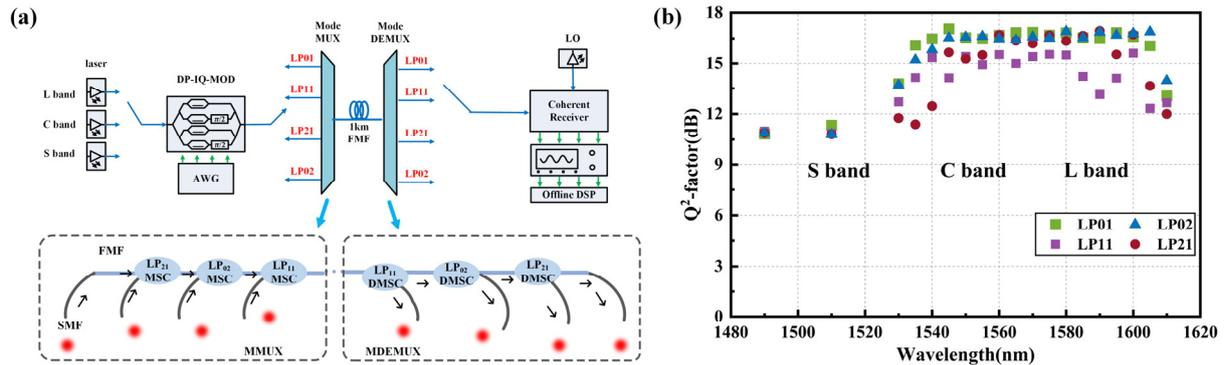
Fig. 3 (a) Experimental setup of transmission. (b) The Q<sup>2</sup>-factor performance after FMF transmission.
