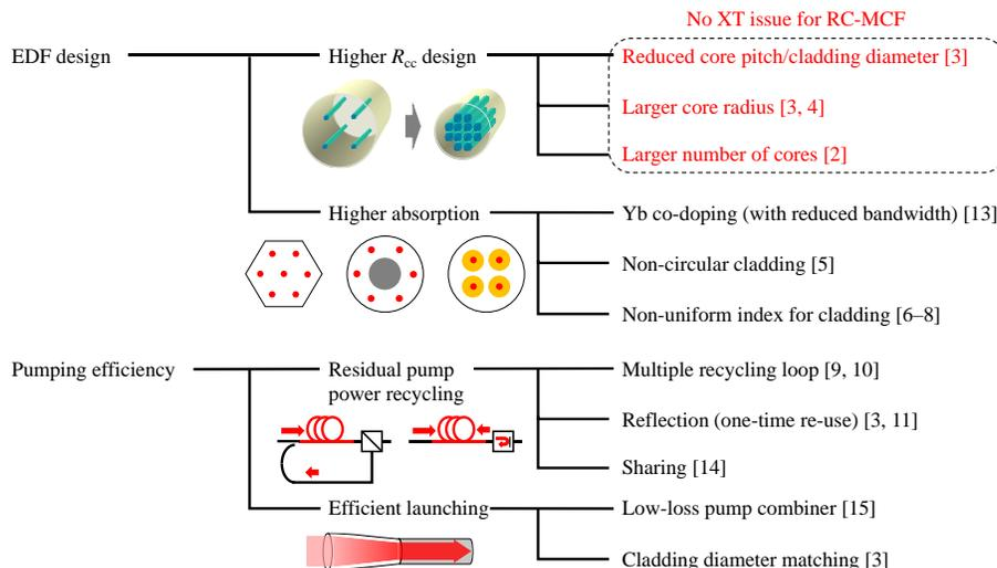
Fig. 1 Latest techniques for improving energy efficiency of cladding-pumped multi-core amplifiers.
