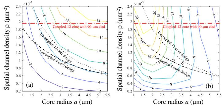
Fig. 3 Power conversion efficiency as functions of core radius and spatial channel density for (a) C-band or (b) L-band single-mode MCF amplifiers.
