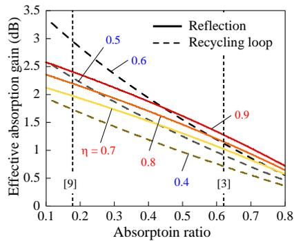
Fig. 4 Calculated effective absorption gain vs. absorption ratio of EDF for reflection (solid) or recycling loop (dashed) configuration.
