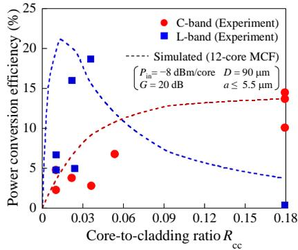
Fig. 2 Power conversion efficiency vs.  $R_{cc}$  of reported C- or L-band SDM amplifiers.
