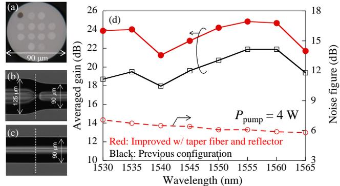
Fig. 5 (a) Cross-section of fabricated 12-core EDF and side-views of splice points between passive fiber and EDF (b) without or (c) with taper fiber. (d) Measured gain and noise figure spectrum of 12-core EDF.
