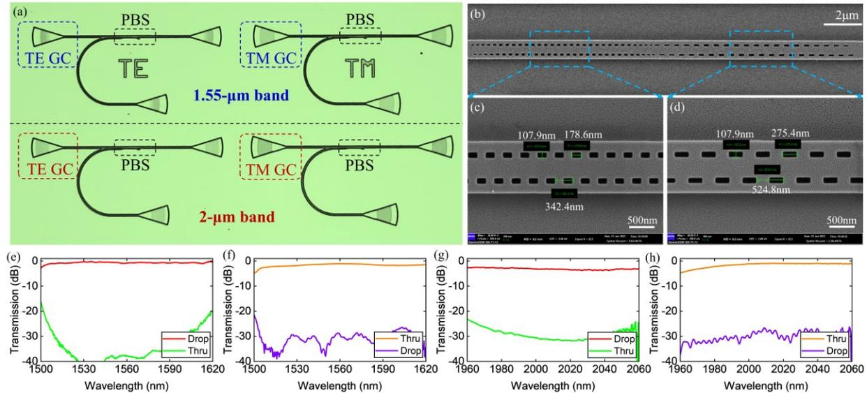
Fig. 3 (a) Microscopic image of fabricated four set devices for measurement. (b) Scanning electron microscope image for MASABG I and II. The enlarged views of UBG in MASABG (c) I and (d) II. Measured transmission spectrum for (e) 1.55 $\mu$ m waveband TE polarization, (f) 1.55 $\mu$ m waveband TM polarization, (g) 2 $\mu$ m waveband TE polarization and (h) 2 $\mu$ m waveband TM polarization.
