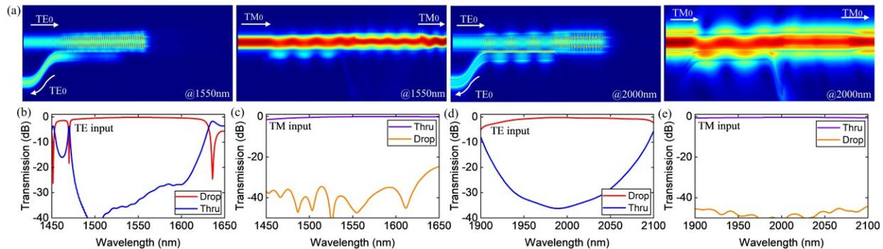
Fig. 2 (a) Light propagation profile for  $\text{TE}_0/\text{TM}_0$  modes at wavelength of 1550/2000nm. Calculated transmission spectrums when (b) 1.55 $\mu\text{m}$  waveband  $\text{TE}_0$  mode, (c) 1.55 $\mu\text{m}$  waveband  $\text{TM}_0$  mode, (d) 2 $\mu\text{m}$  waveband  $\text{TE}_0$  mode and (e) 2 $\mu\text{m}$  waveband  $\text{TM}_0$  mode is launched.
