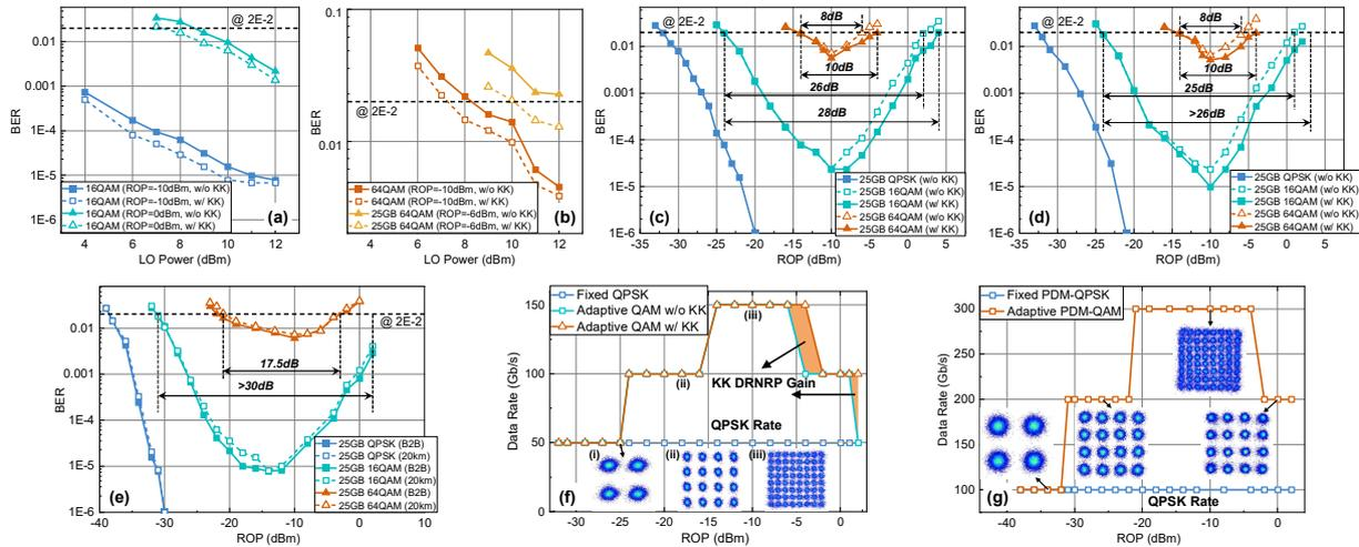
Fig. 3 (a) BER versus LO power for Alamouti-coded 16QAM. (b) BER versus LO power for Alamouti-coded 64QAM. (c) and (d) show BER versus ROP for ultimate-simplified coherent Rx in B2B and fiber transmission cases. (e) BER versus ROP for full coherent Rx. (f) and (g) illustrate the data rate under different schemes in the total dynamic range for simplified coherent Rx and full coherent Rx, respectively.
