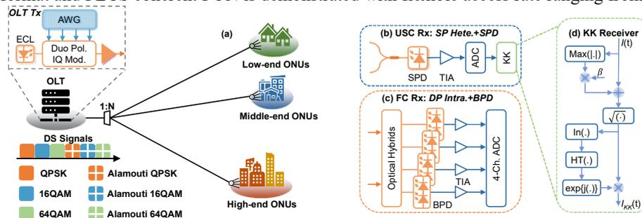
Fig. 1 (a) An example of future downstream TDM-PON system with different types of coherent receivers. (b) and (c) are the ultimate-simplified coherent receiver and full coherent receiver. (d) Diagram of KK receiver.
