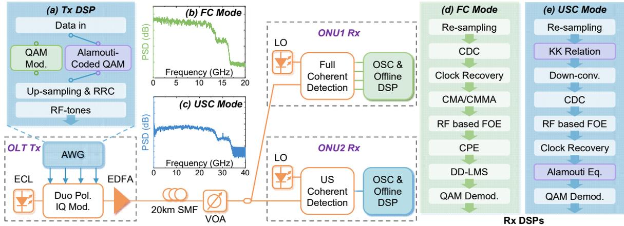
Fig. 2 Experimental setup of the downstream hybrid FLCS-CPON system. (a) the Tx DSP. (b) and (c) are the electrical spectrum after full coherent and ultimate-simplified coherent detection, respectively. (d) and (e) are the Rx DSP for these two types of coherent receivers.
