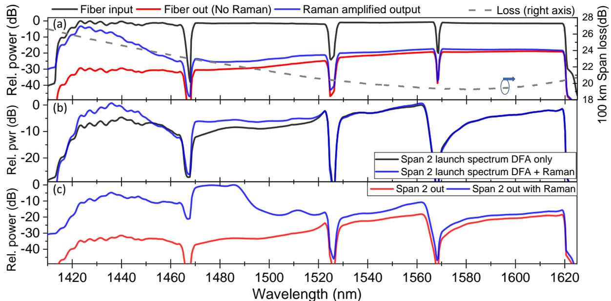
**Fig. 2:** Wideband signal spectra (a) left-axis E/S/C/L-band signal at input (black) + output (red) of first fiber span with Raman amplification profile (blue). Right-axis span loss of 100 km fiber span, (b) Launch spectra after mid-stage DFA amplification with and without Raman pumps acting on first span, and (c) output of span 2 with and without Raman amplification in both spans.
