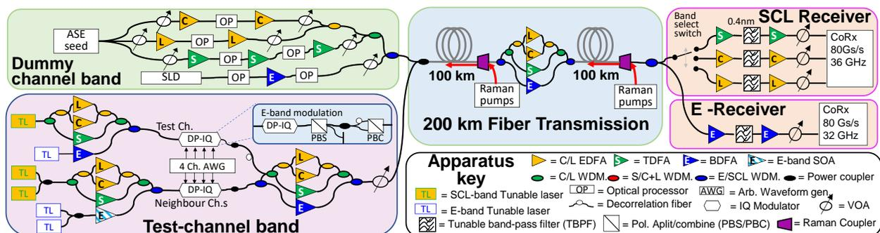
Fig. 1: (a) Experimental set-up for E, S, C + L-band transmission
